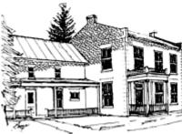
Constructed as a store and furniture factory by cabinet maker John Mills. Note the parapetted end gables to hel prevent spread of roof fires to neighbours.
